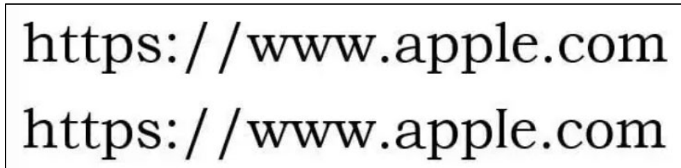
Figure 2: Example of a homograph attack by swapping out the "l" in Apple for a "1" or a lowercase "L" (Source: Identity Guard)
